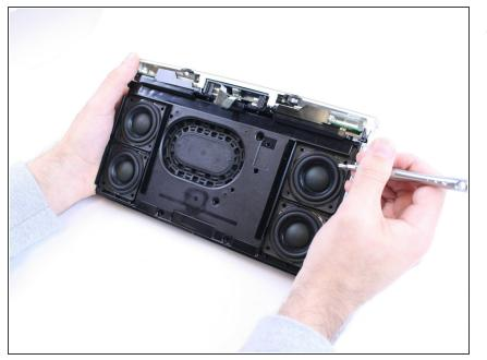
There are four T-10 Torx screws for each speaker; remove all four screws for each speaker you are replacing.
