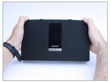
Grip the sides of the device and push the speaker grille down and out.
