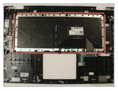
Unscrew & remove the sixteen 2mm screws holding the keyboard (using a PH000 screwdriver bit)
