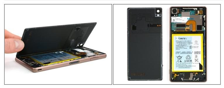
After pulling out the adhesive tabs, you can lift the back cover and remove it.
