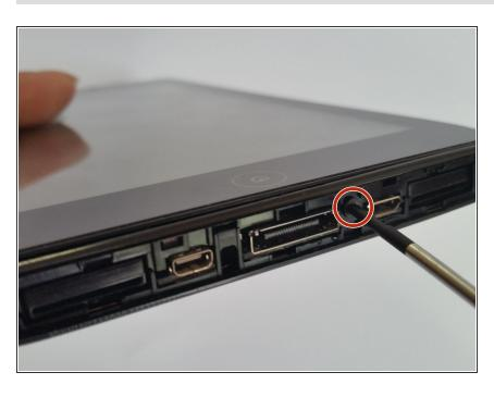
Remove the five 4 mm screws from the edges of the tablet with a Phillips #00 screwdriver.
