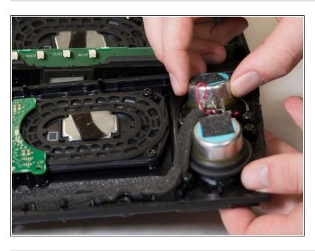
Carefully pop out the speaker after the wires have been unwound.
