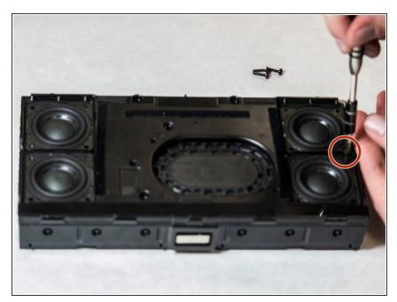
Using the T-10 star tip screwdriver, unscrew the four 13 mm screws around each of the speakers.
