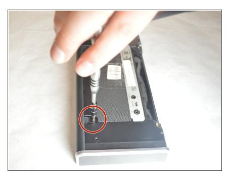
Once the Bose Soundlink II Side Covers Removal has been completed, remove the two screws (13 mm) an inch below the buttons on the back of the speaker using the T-10 star tip screwdriver.
