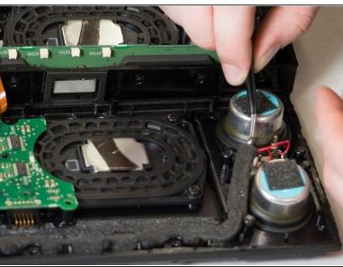
Unwind the wires corresponding to the speaker you want to remove (our photo shows the removal
