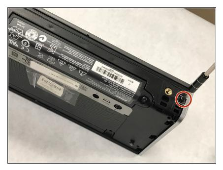
Using the T-10 star tip screwdriver, remove the two 13 mm screws located on the bottom of the speaker on each side of the battery pack.
