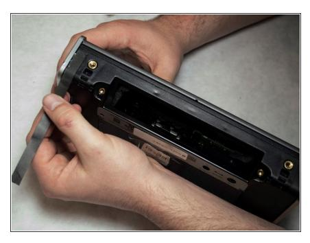
Remove the black electrical tape in order to reveal the screws attaching the side cover to the main body of the speaker. These screws are on the base of the device.
