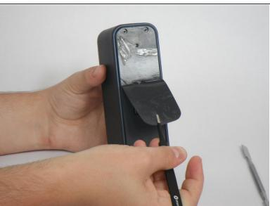
Using a plastic opening tool, go around the edges of the rubber bottom. Insert the same tool under the edge of the rubber and swivel side to side. Continue moving it forward while peeling the plastic off with the precision tweezers.
