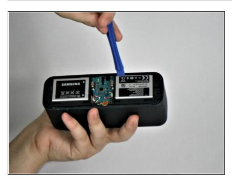
Using the plastic opening tool, remove the batteries from the device.
