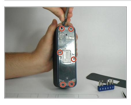
Remove the six 4.5 mm Philips #1 screws from the bottom plate using the Screwdriver J00. Take off the bottom plate.
