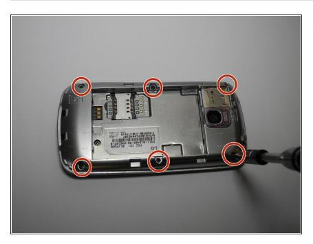
Use a J0 screwdriver to remove the six 4.5mm screws.
