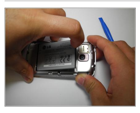
Remove the battery. There's an indentation to the left of the camera lens to pull up on the battery with your finger
