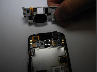
Remove SD card mount. Insert the plastic opening tool on the right side to pop off
