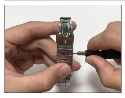
Remove pin from watch band link to obtain easier access to the back of the watch.
