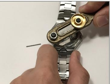
• Using the adjustable wrench, unscrew the back face of the watch.
