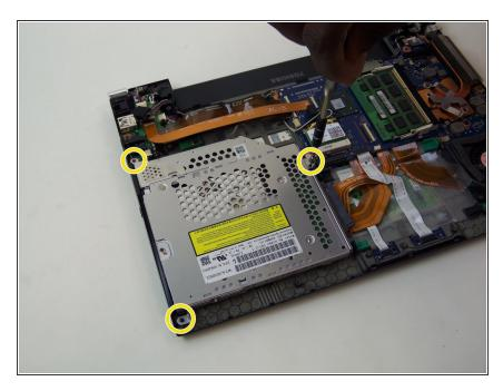
After the cover is removed, remove the screws that hold the Drive. It has 3, 1 cm screws holding it down.
