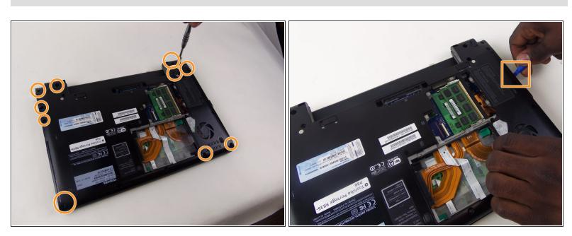
Start by removing the back cover by removing the screws, revealing the Optical Drive. Remove the
