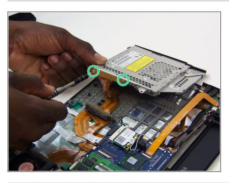
Take the 2, .5 cm screws out of the drive line. Once this is complete, you have successfully taken out the Optical Drive.
