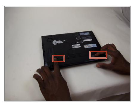
Start by removing the battery.
