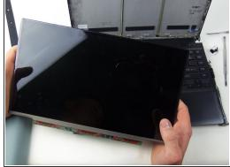
Remove the cord from the screen by cutting the tape where the two fittings meet. After that pull them apart.
