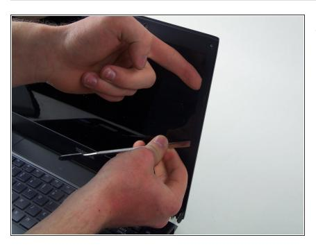
Remove the plastic bezel by lightly prying on it. It will pop when it starts to come loose.
