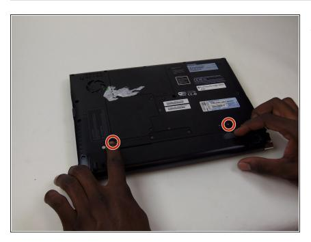
Remove the battery by pressing the two buttons inward and pulling the battery out.
