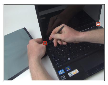
Remove the end caps located on the left and right corners below the screen.
