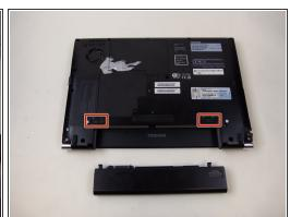
Remove the battery by sliding the interlocks to the unlock position.
