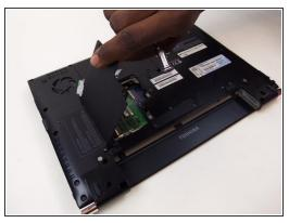
• Remove the two 6mm screws from the RAM cover. Lift the RAM cover upward to remove.
