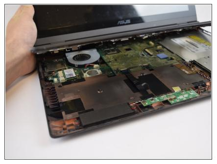
• Carefully lift and remove the plastic cover to avoid damaging anything.
