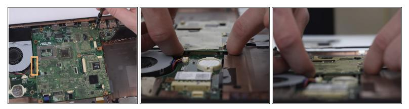
• Lift the Motherboard with your fingers by reaching underneath the Motherboard and prying.
