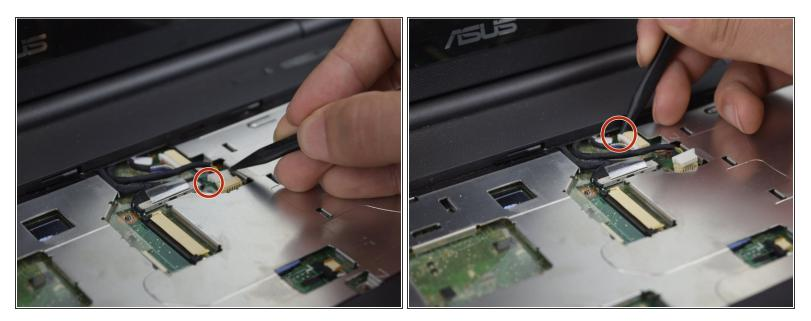
Use the spudger tool to unplug the two cords from the body by pushing on the tabs on both sides of the plug.
