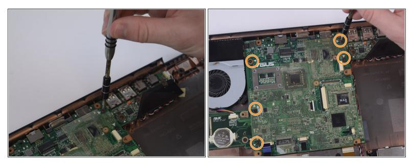
Remove the five 4 mm Phillips head 5 mm long screws that have white arrows pointing to them with the screwdriver.
