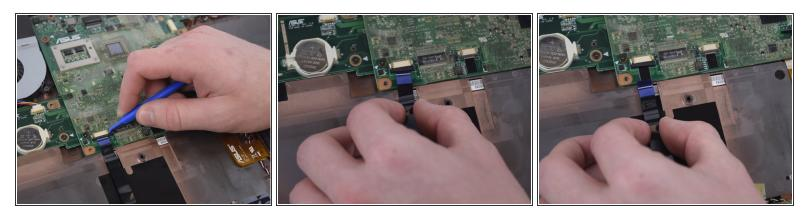
• Use the Plastic Opening Tool to unplug the blue cord on the Motherboard.
