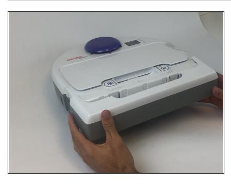
Pull the left and right sides away from the machine to unclip the bumper. This requires that you bend the plastic a little bit. Unclip one side a little bit and allow the prong to rest on the side of the machine. Then unclip the other side and pull off the bumper parallel to both sides
