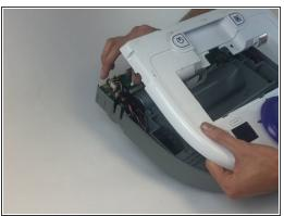
To remove the top, you must press in both of the clamps at the same time and push upwards.
