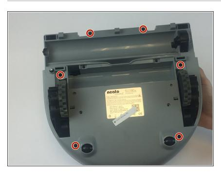
Begin by placing the robot on it's back and removing the six 11m screws using a Torx T10 screwdriver.
