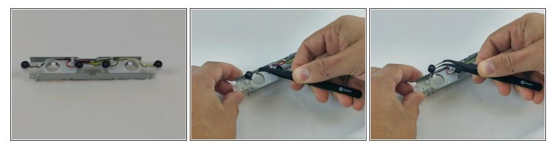
Using fine point tweezers, grab hold of each microphone, one at a time, and lift from the plastic frame.
