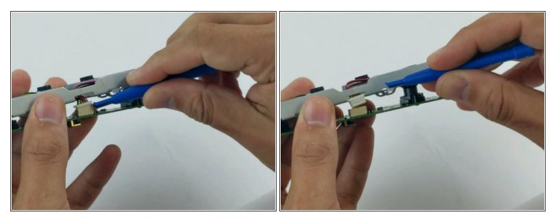
• Using a plastic opening tool, disconnect the microphone array connector from the motherboard.
