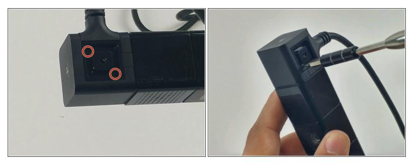
• With the PH000 sized screwdriver, remove the two 6.5mm Phillips #000 screws located under the stand connection point, where the cable enters the case.
