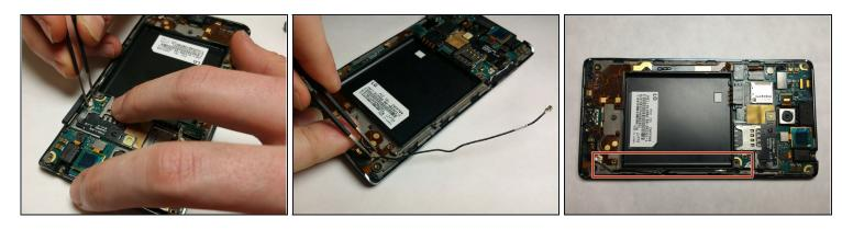
Remove both connections of the antenna by pulling up with tweezers
