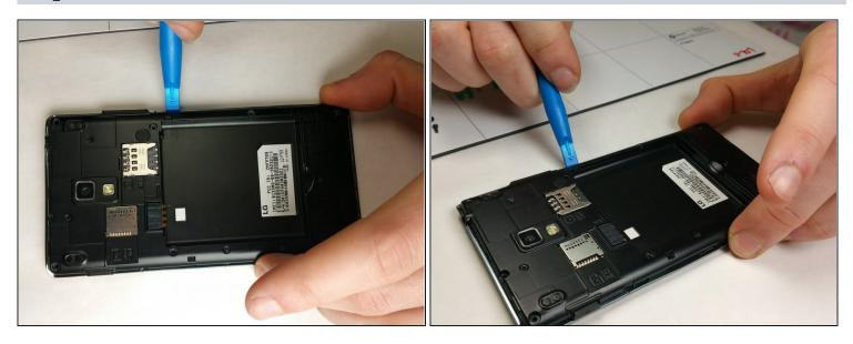
Using a small prying tool, carefully remove the back frame by prying on the sides of the device.
