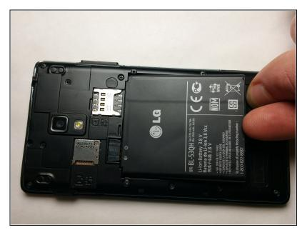
Lift and remove the battery from the notch in the edge of the battery compartment
