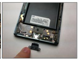
• Remove Micro-USB Cache by unscrewing both 2.9mm screws with the PH000 headtype
