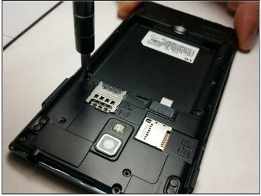
• Remove all 10 of the 4.5mm screws that hold the back frame to the case of the phone using a PH000 screwdriver.
