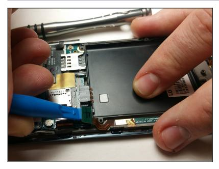
Detach module from motherboard using a prying tool
