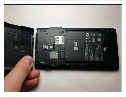
Power off the device and gently lift the battery cover off to access the battery
