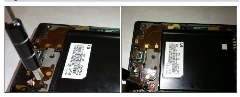
• Remove 1.8mm screw to free Micro-USB module for removal using the PH000 headtype
