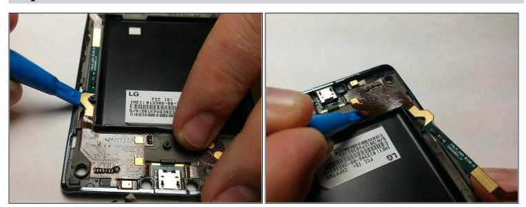
• Use a small prying tool to detach the Micro-USB circuitry from the case of the phone
