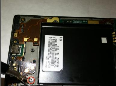
Remove 1.8mm screw to free Micro-USB module for removal using the PH000 headtype
