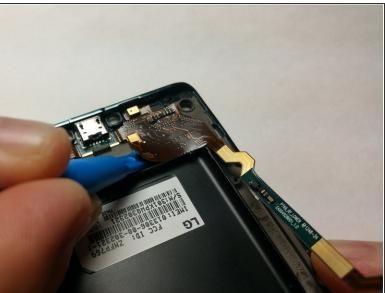
Use a small prying tool to detach the Micro-USB circuitry from the case of the phone
