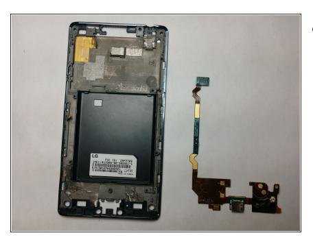
Comparison showing the Micro-USB module against the empty phone casing
