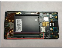
Remove both connections of the antenna by pulling up with tweezers
