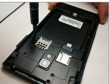
Remove all 10 of the 4.5mm screws that hold the back frame to the case of the phone using a PH000 screwdriver.
