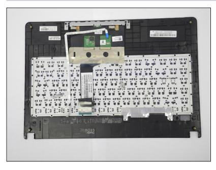
Lay the keyboard cover down with the keys facing down. This component contains the track pad. You will be working with this component until you reassemble.
