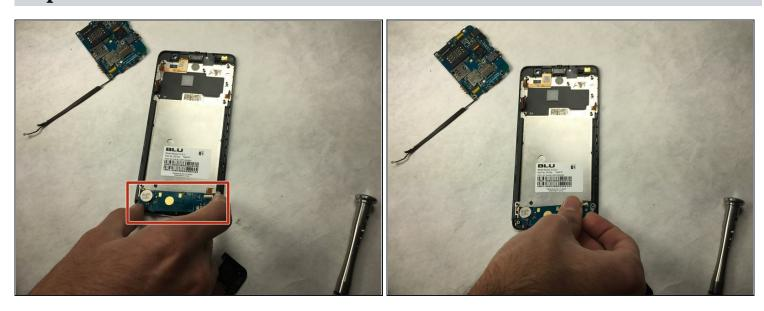
• Peel off the bottom back with finger or supdger.
