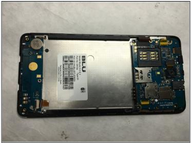
• Remove the bottom inner back plate.
