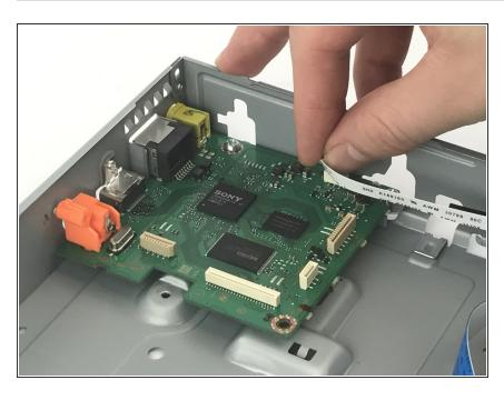
Remove the ribbon connecting the Wi-Fi module to the motherboard.
