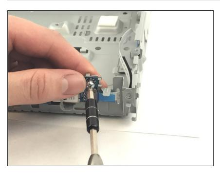
Use the PH1 screwdriver to remove the 7mm screw on the module.
