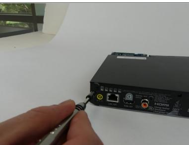
Use the PH1 screwdriver to remove the two 9mm screws on the back of the Blu-ray player.
