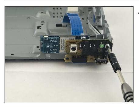
Use the PH1 to remove the 7mm screw on the port board.
