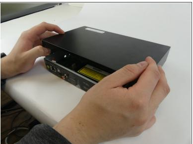
Remove the back of the device by slowly sliding the rear outer housing backwards.
