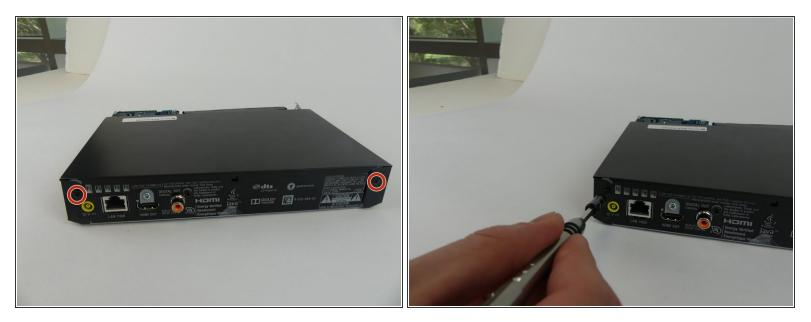
• Use the PH1 screwdriver to remove the two 9mm screws on the back of the Blu-ray player.
