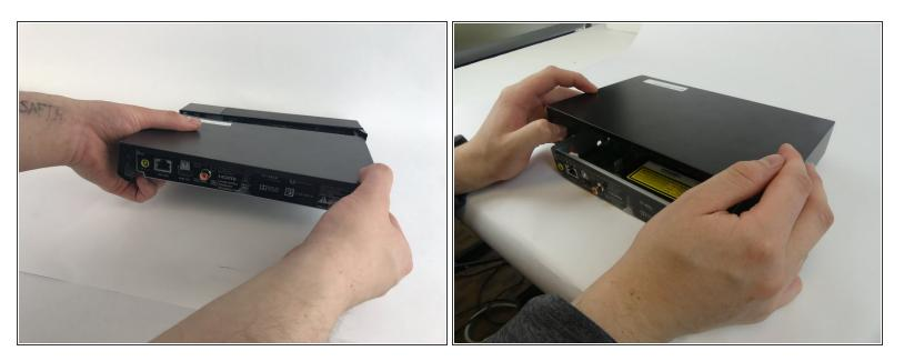
• Remove the back of the device by slowly sliding the rear outer housing backwards.
