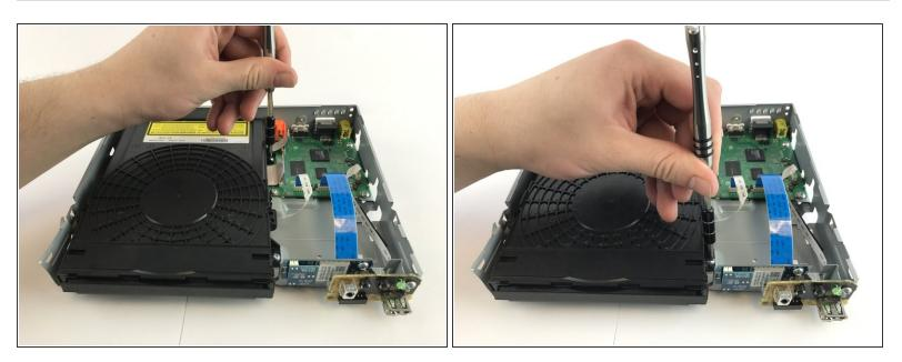
• Use a PH1 screwdriver to unscrew both of the 7mm screws on the side of the disc reader.
