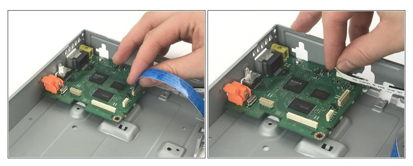
Gently pull upwards on the ribbon cables to disconnect the motherboard from the Wi-Fi module and port board.
