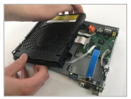
• Gently slide the disc drive to the right and lift up to remove the disc drive from the body of the player.
