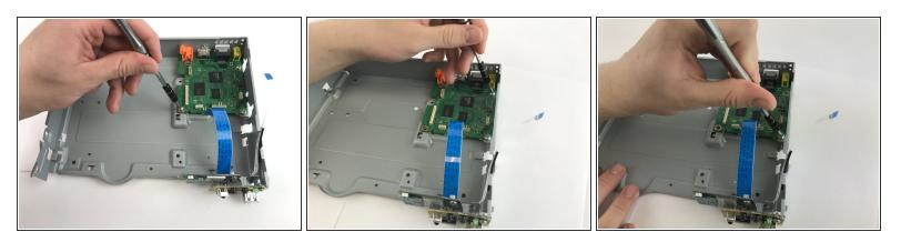
• Remove the three 7mm screws along the motherboard using a PH1 screwdriver.
