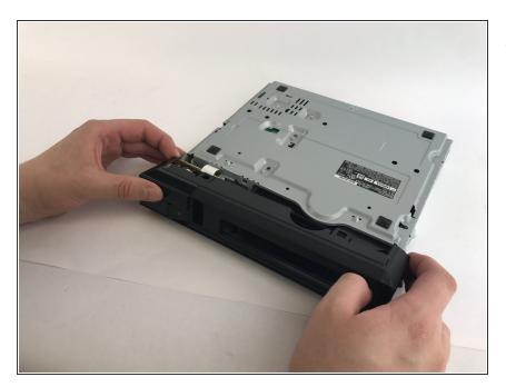
• Once all the clips are open, slide the front outer housing out.
