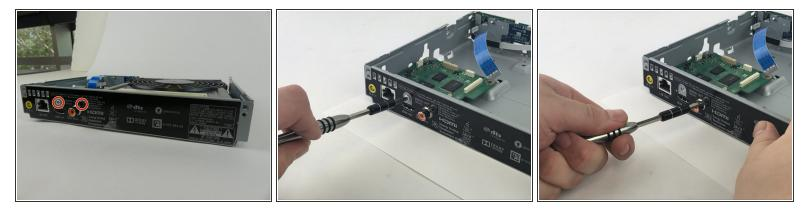
Remove the 4mm screw above the HDMI port and the 9mm screw Digital Out port.
