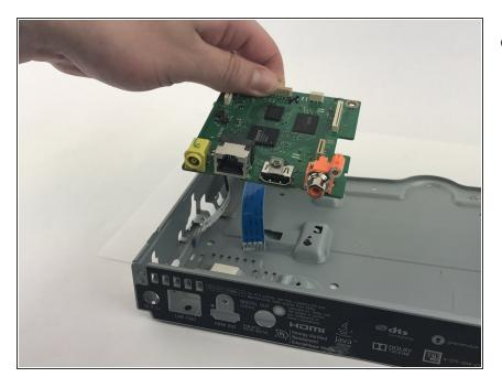
• Carefully lift and pull the motherboard forward to remove.
