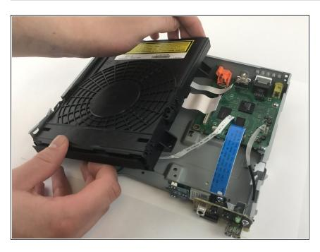
Gently slide the disc drive to the right and lift up to remove the disc drive from the body of the player.
