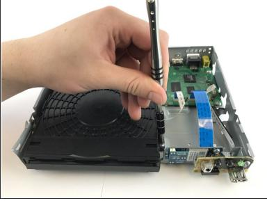
Use a PH1 screwdriver to unscrew both of the 7mm screws on the side of the disc reader.
