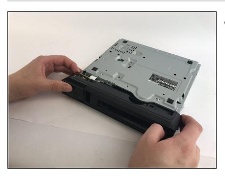
Once all the clips are open, slide the front outer housing out.
