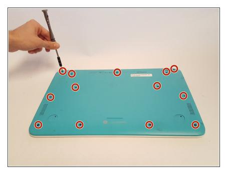
Using a Phillips #1 screwdriver, remove the thirteen 5.7 mm screws located on the back of the device as shown.
