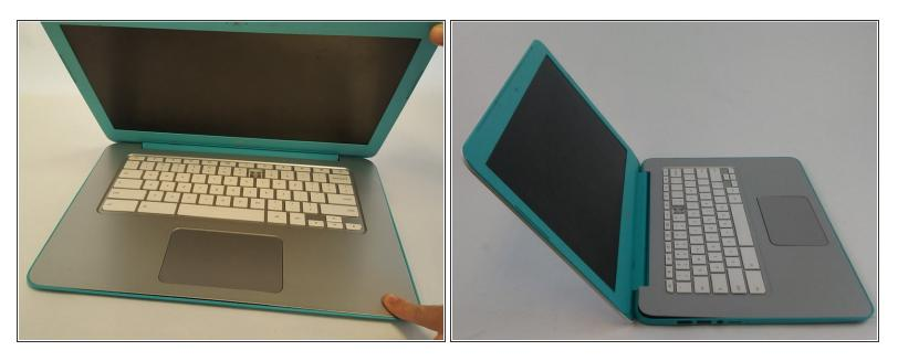
Carefully open the computer's lid as far as it will go until the back edge of the keyboard cover separates from the base.
