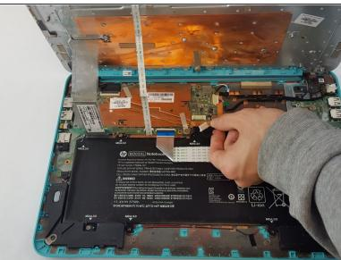
Using a spudger, remove the battery cable by slowly pulling the plastic connector towards you.
