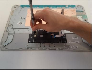
Using a Phillips #000 screwdriver, remove the two 2.4 mm screws that secure the TouchPad to the keyboard cover.
