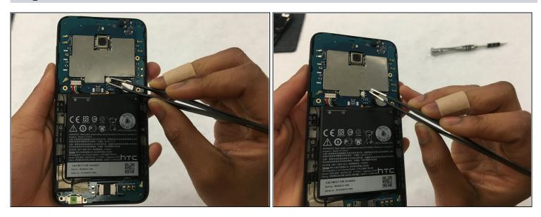
• Pull the wire harness from the circuit board that is connected to the vibration motor using a pair of precision <u>tweezers</u>.
