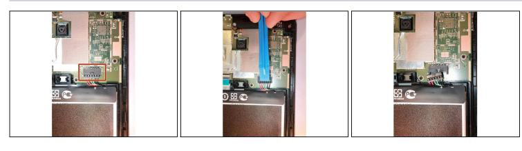
• Use an iFixit opening tool to gently push the black bundle cable connector in a forward motion until it loosens without pushing down on the bundle cable connector.
