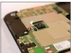
• Use a plastic opening tool to push the white cable connector out of its port in a side to side motion.
