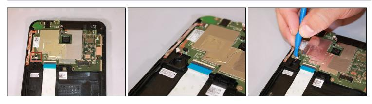
• Use a plastic opening tool to slide the white cable connector completely out of the port.
