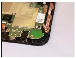
• Use the wide nosed tweezers to gently pull out the orange ribbon inserted in the port on the motherboard.
