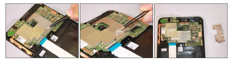
• Remove the silver tape on one corner with the needle nosed tweezers, and remove the tape from the motherboard.
