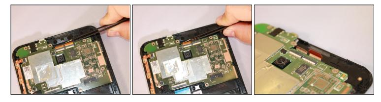
Use the needle nosed tweezers to gently pull both of the orange ribbon cables out of their ports.
