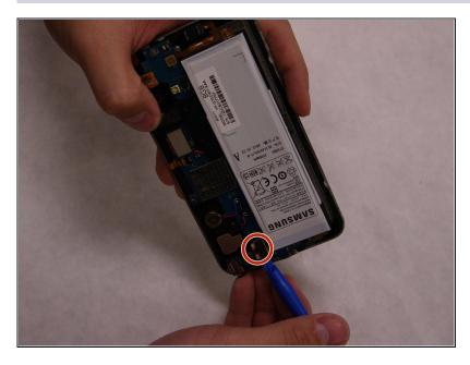
Use the pry tool to separate the tab connecting the battery and motherboard.
