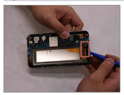
Remove the ear piece using a pry tool. Set aside.
