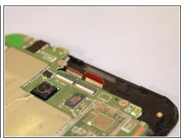
Use the needle nosed tweezers to gently pull both of the orange ribbon cables out of their ports.
