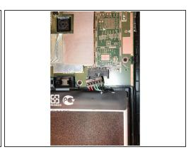
• Use an iFixit opening tool to gently push the black bundle cable connector in a forward motion until it loosens without pushing down on the bundle cable connector.
