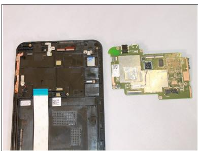
To uninstall the motherboard, use the metal spudger tool to lift it out of the device.
