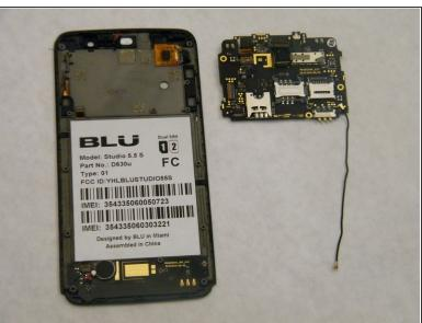
Use the tweezers to grip the bottom of the motherboard and lift up.
