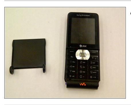
Remove the cover with a slight twisting motion.
