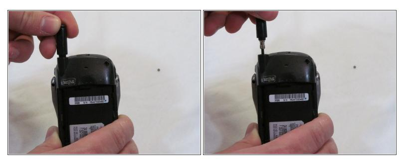
• Grasp the antenna firmly and rotate it counterclockwise to unscrew it from the phone.
