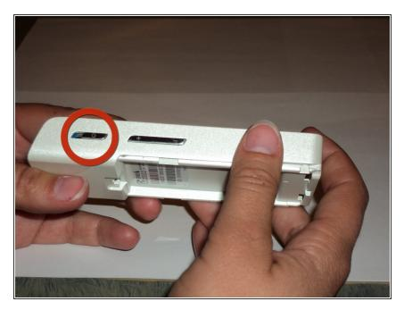
Locate the power button on the side of the device (the power button is circled in orange in the photograph).
