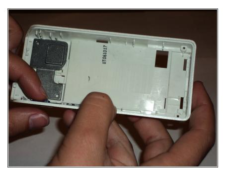
Grasping the button as shown, slide the power button all the way to the right.
