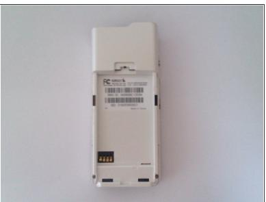
Remove the battery (which also functions as the back cover) from the device. This step is not
