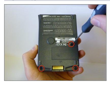
Unscrew the three screws on the back of the Palm Pilot.
