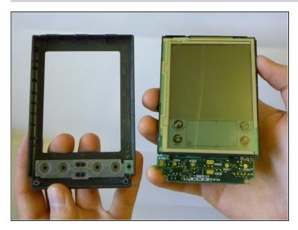
The front plastic cover is now free to be removed from the rest of the device.
