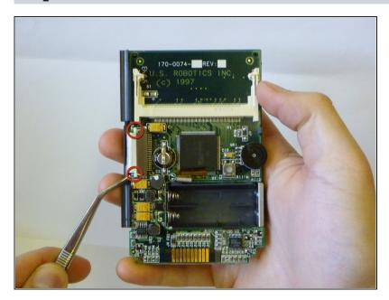
Looking at the back of the device hold one of the white tabs on the ribbon cable connector down and use tweezers to push in the other white tab toward the device at the same time.
