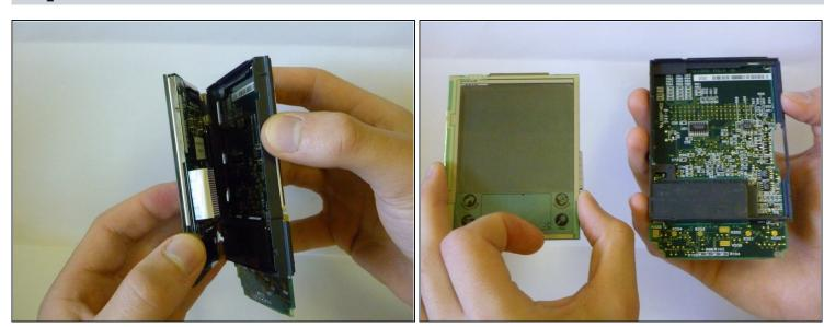
• The screen is now disconnected from the rest of the device and can now be removed.
