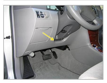
You will find the fuse box behind the coin pocket at the left side (not for uk models). Open the coin pocket and then pull it off. You will see fuses in the hole. It is a black covered square box inside - usually press the sides and the cover should pop off. For UK, passenger side, open the glove box, pull it off clip hinges, box is behind.
