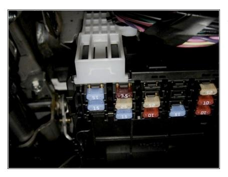
After taking the box cover you will be able to change the fuse. In my case it was the number 38 (in the fielder model the position can change). For more details see the User's Manual for fuse diagrams.
