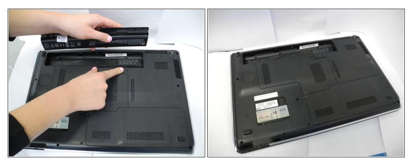
• Carefully pull out the battery while holding the latch to the open position with your finger.
