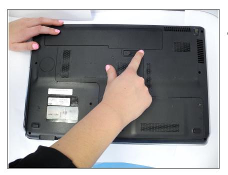
• Slide the battery latch to the left to release the battery.
