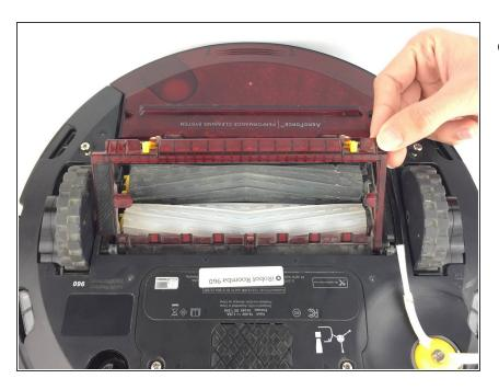
Lift the frame to expose the two debris extractors.
