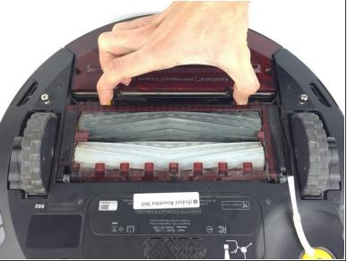
• Pinch the two yellow tabs that are located near the dustbin towards each other to open the frame.
