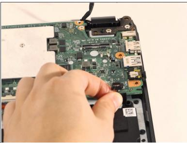
Locate the cable that attaches the speakers to the motherboard. Unhook the cable.
