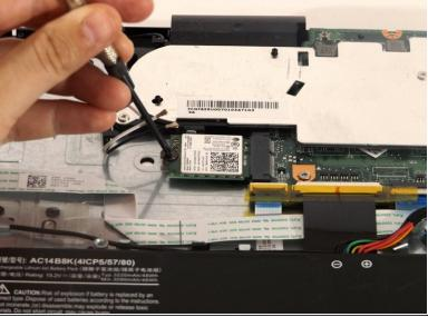
Locate the screw that holds the wireless card in place and then remove it using a screwdriver with a PH0 bit.
