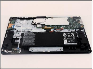
Using a spudger, gently pry open the back from the top.
