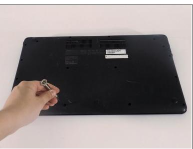
Remove the 18 Phillips screws using a screwdriver with a PH0 bit.
