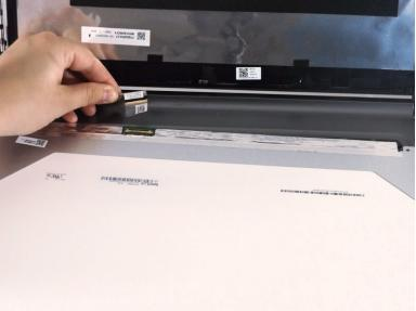
Remove the LCD data cable which will allow the screen to be removed completely.
