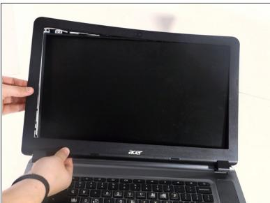
Remove the bezel with a plastic spudger.
