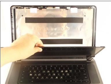
Remove Screen by gently pulling it out and then lifting it up.
