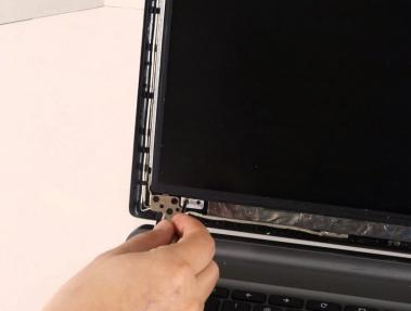
Remove four screws - one in each corner along the screen.
