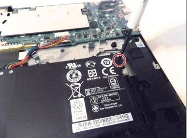
Next, unscrew the battery pack. The one screw should be located on the far right of it. This will
