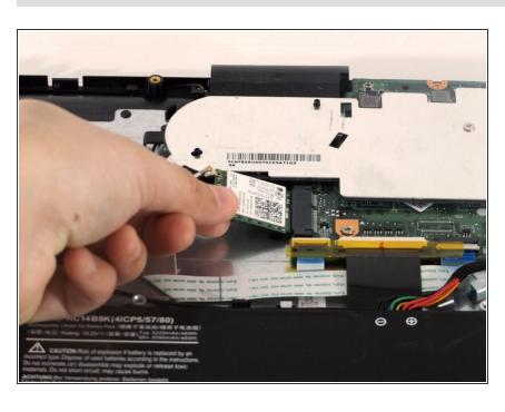
Slide the Wireless card out gently with two fingers while being careful not to damage any surrounding parts.
