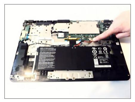
Once it is opened up, locate the battery and the cable that is attached to it.
