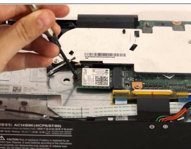
Locate the screw that holds the wireless card in place and then remove it using a screwdriver with a PH0 bit.
