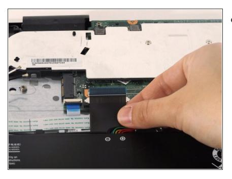
Remove the large black cable between the two ribbon cables.
