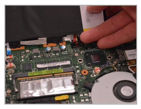
• Unclip the battery terminal by prying straight up on the sides of the connector to release the clip.
