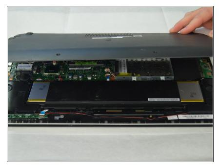
• Remove the back plate by lifting it straight up.
