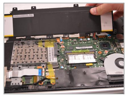
• Lift up the battery to reveal the battery terminal.
