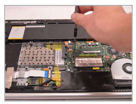
• Remove 9 (.5 cm) phillips screws around the edge of the battery.
