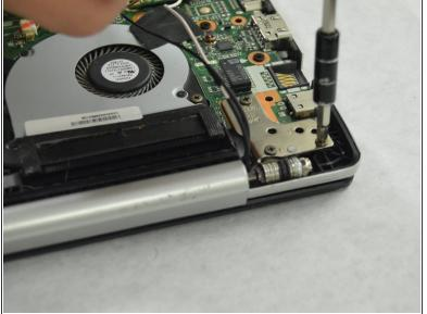
Remove 3 (.5 cm) phillips screws around the edge of the hinge. Repeat for other side.
