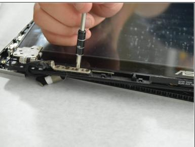
Remove 4 (.5 cm) screws from the hinge. Remove the hinge and follow steps in reverse order to reassemble and complete repair.
