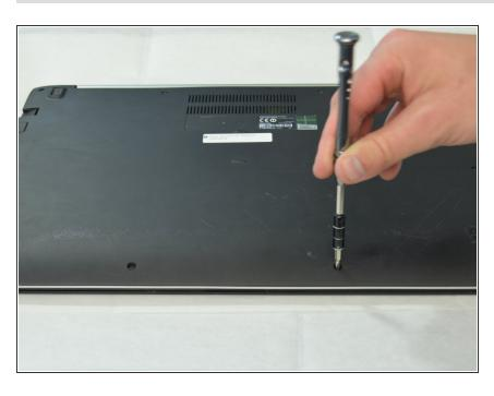
Use a Philips Head PH1 screwdriver to remove 10 screws (3 10mm screws and 7 5mm screws) around the perimeter of the back plate.
