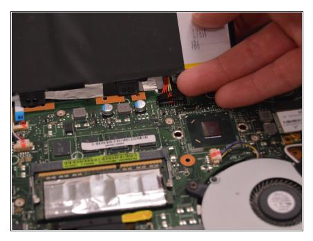
Unclip the battery terminal by prying straight up on the sides of the connector to release the clips.
