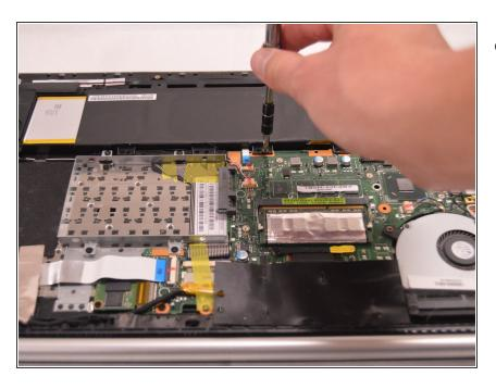
Remove 9 5mm screws around the edge of the battery
