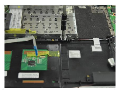
Remove 2 5mm screws from the hard drive casing.
