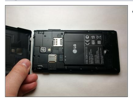
Begin the process with the device face down to remove the back cover. Remove the battery cover using your hands to access the inside of the phone.
