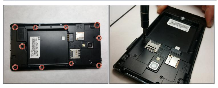
Use Philips PH000 to remove 10 screws located on back of device near the edges.
