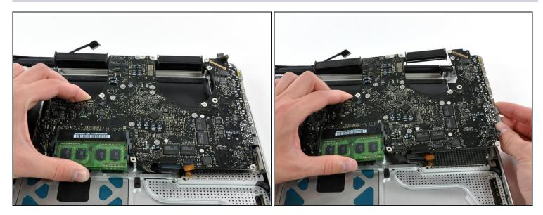
• Carefully lift the logic board assembly from the left side and work it out of the upper case, minding the port side that may get caught during removal.
