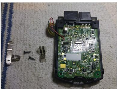
Remove the two battery terminal screws
