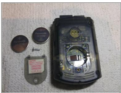
Remove the silver screw and batteries
