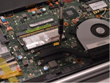
Remove 2 (.5 cm) Phillips Head screws found around the fan and 4 (.3 cm) Phillips Head screws found around the heat sink connector.
