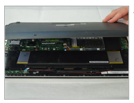
Remove the back plate by lifting it straight up.
