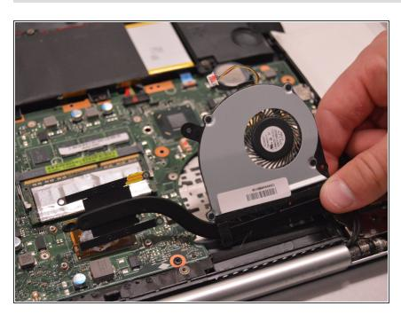
Remove the fan and connected heat sink by lifting straight out of the assembly.
