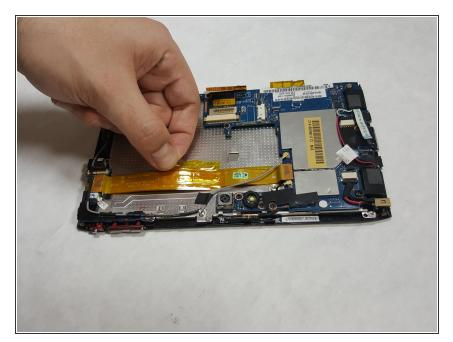
Gently peel off any tape securing the FPC to the main plate.
