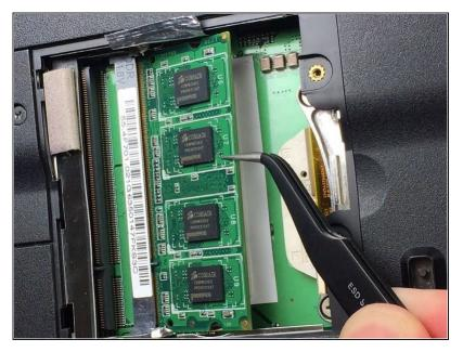
Repeat Step 5 and use tweezers to carefully pull RAM away from RAM slot
