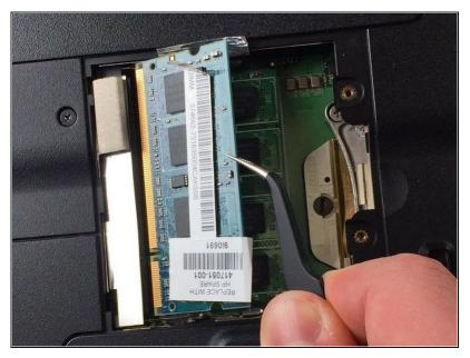
Using <u>tweezers</u>, carefully pull the RAM chip away from the RAM slot
